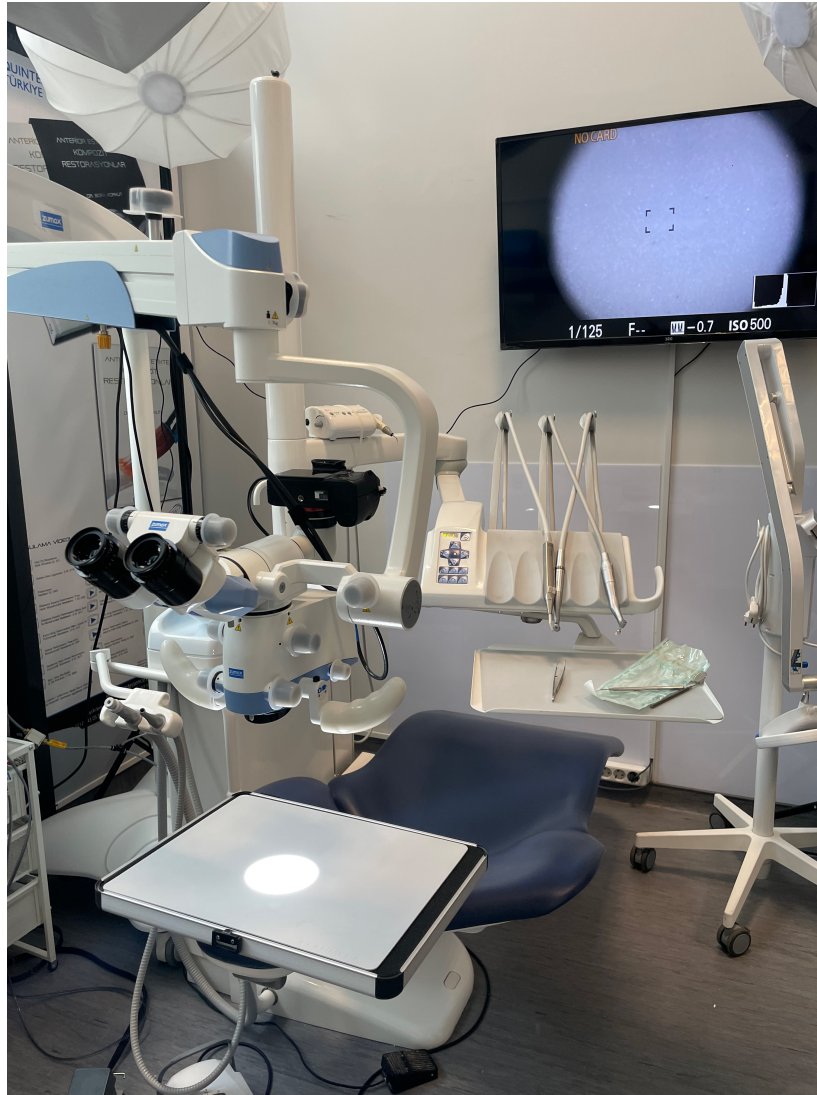
FIGURE 2. Stereomicroscope setup used for surface evaluation. Photograph of the stereomicroscope setup used to document post-aging surface texture at 30 \times magnification. The setup was used to examine the brushed and protected reference halves of each specimen.
