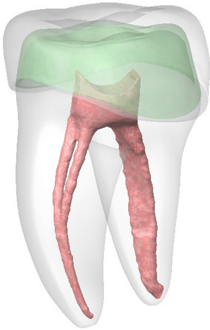
FIGURE 1. Solid model of the prepared tooth, pulp chamber, cement layer, and prefabricated crown.
