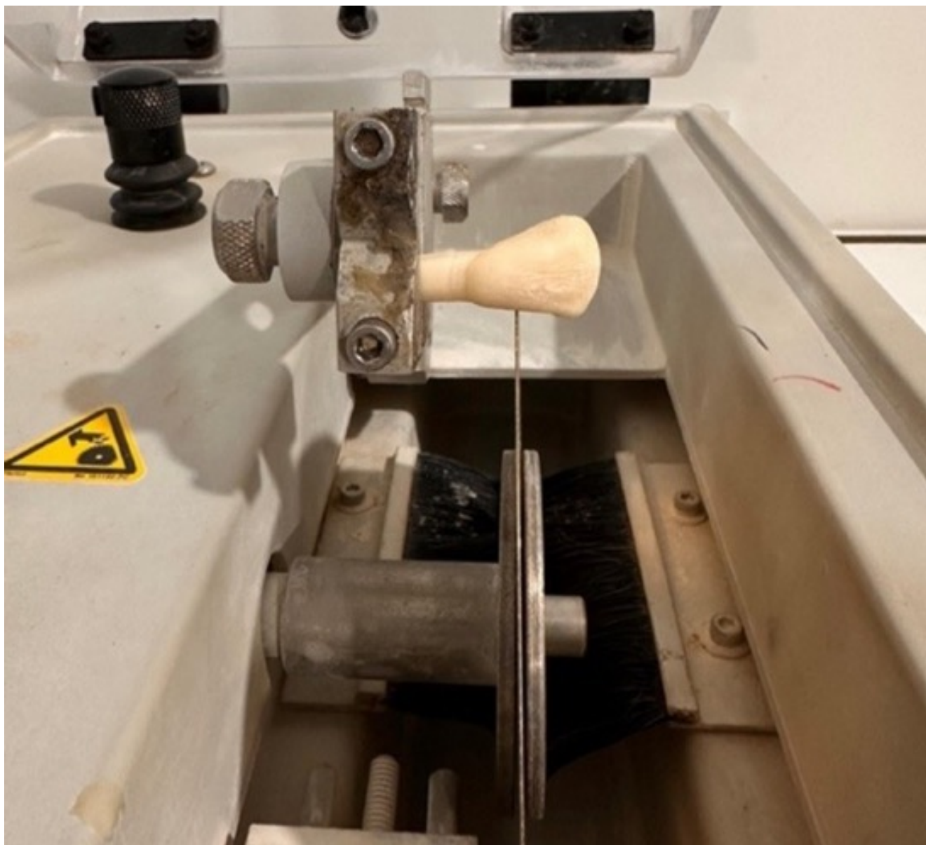
FIGURE 1. The separation of the teeth from their roots using a precision saw (BUEHLER IsoMet® 1000) and a diamond separator (A7354 Medium Grain 200, 0.17 mm Acurata®) under water cooling.
