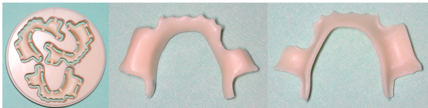
FIGURE 4. Manufacturing of the pediatric partial denture using subtractive manufacturing.
