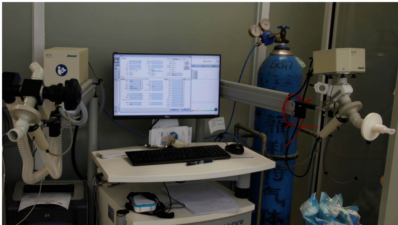
FIGURE 1. MasterScreen PFT System, pulmonary function instrument (CareFusion, Germany). Technical parameters: (1) Flow rate capacity sensor (high-quality digital) (range 0 \pm 20 L/s, accuracy (0.2\text{--}12) L/s ( \pm 2\% ), resolution 10 mL/s, resistance <0.05 kPa/L/s); (2) Capacity (built-in software with digital integration method analysis) (range 0–20 L, accuracy (\pm 50 mL, \pm 3\% ), resolution 1 mL); Several supporting mouthparts, and 1 desktop computer.
