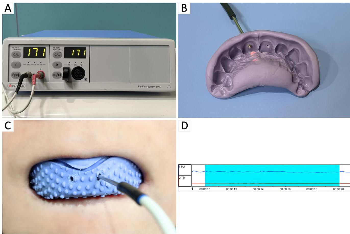
**FIGURE 4. Dental pulp blood flow data collection process.** (A) Laser doppler flowmetry device. (B) Fabrication of a silicone rubber guide. (C) The testing process. (D) Results of dental pulp blood flow. PU, Perfusion Unit; TB, Total light Back.
