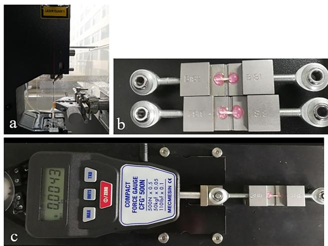
**FIGURE 1. The experimental process of the study.** (a) Hard tissue slicer. (b,c) Micro-tensile strength test.
