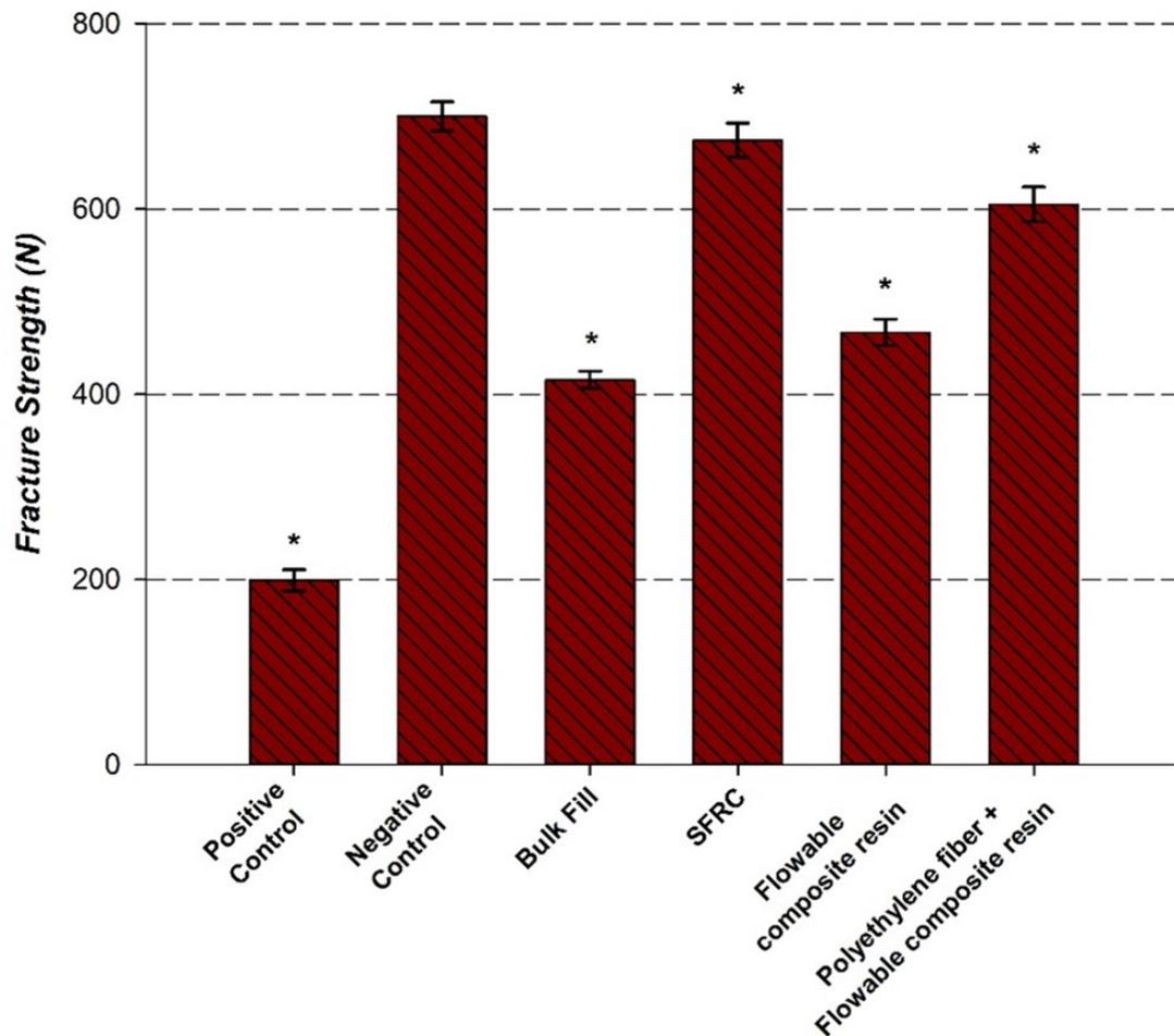
**FIGURE 3. The values of the fracture strength of all the sample groups.** \*shows a statistically significant difference in fracture strength among the groups. SFRC: short fiber reinforced composite.
