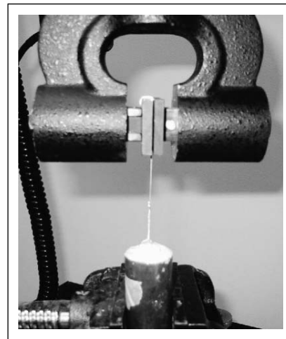
Figure 2. Shear Bond Strength Test
