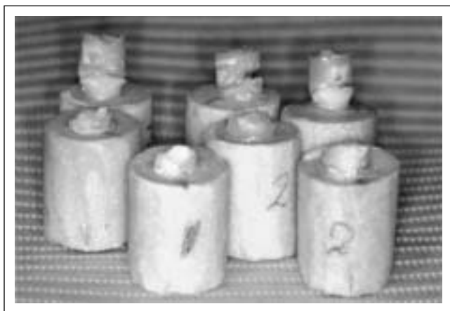
Figure 4. Specimens after applying the fracture load. A complete fracture is evident in groups I & II where no fibre post was inserted. Cracking and incomplete separation of the crown occurred in samples where a fibre core was inserted.
