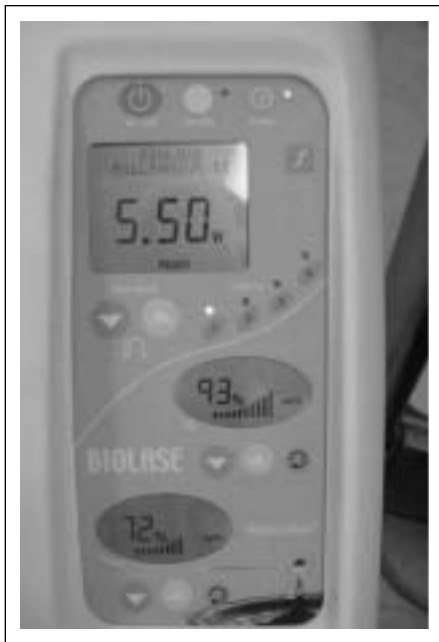
Figure 1. Setting to cut Enamel uses power.
