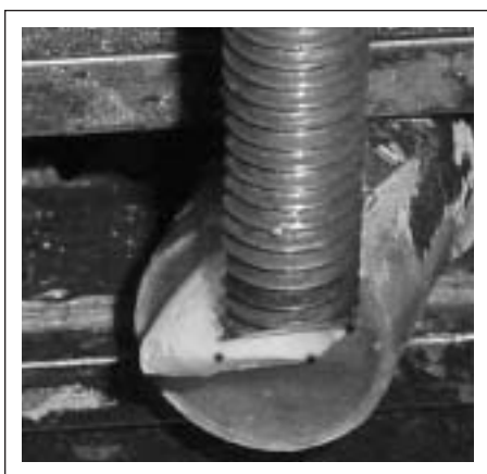
Figure 6. Position of the Instron crosshead on the restoration.
