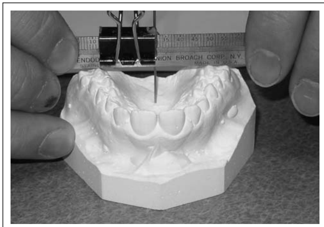
Figure 1. Photograph of the device to measure the height of palates. The binder clip holds a tube through which is inserted a piece of orthodontic wire. The wire is measured from the level of the ruler to the palate.
