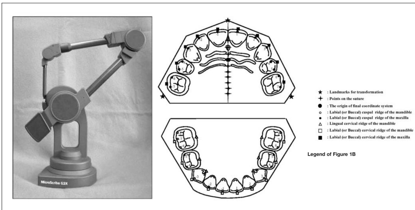
**Figure 1.** (A): the measuring device (Microscribe G2X) used in this study. (B) Digitized points 1) for the transformation of the coordinate system (★), 2) to make standard plane (△), 3) to generate the anterior-posterior axis (\*), 4) for the origin of system (●), 5) to make dental arch form (numbering as “t” in the text) (○), and 6) to measure buccal height (■).
