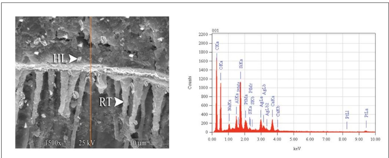
**Figure 2.** EDS spectrum for Prime & Bond NT (Group A)
