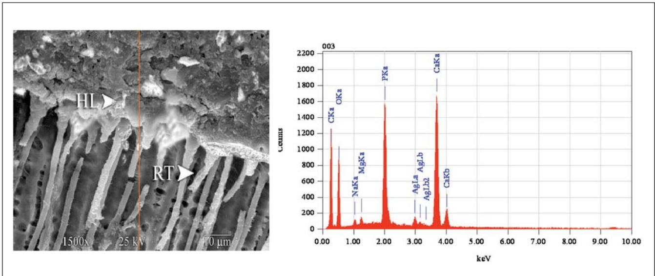
Figure 4. EDS spectrum for AdheSE (Group B)
