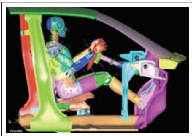
Figure No. 4. Finite element analysis for crash testing
