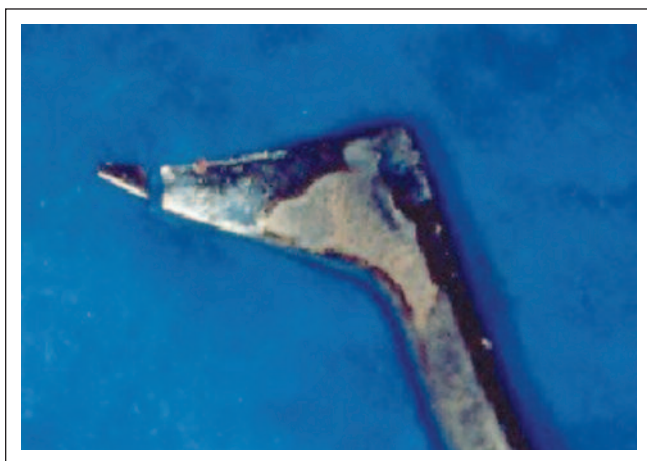
Figure 2. Broken elevator and its matching fractured piece.
