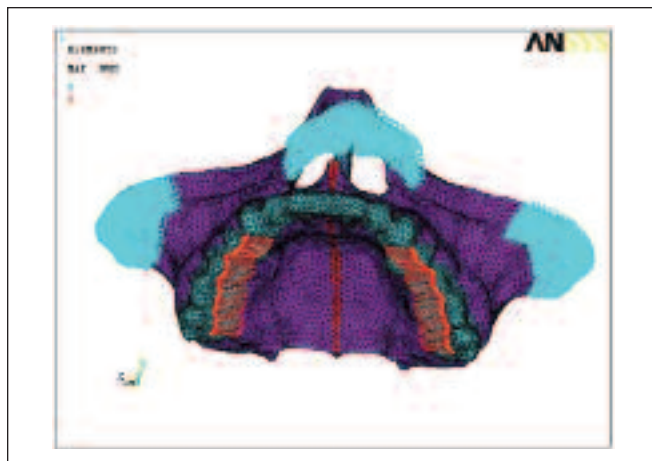
Figure 1. Finite element model of maxilla with boundary conditions assigned—The boundary conditions in the finite element model basically represent the load imposed on the structures under study and their fixation counter parts. The points at the frontal process and the zygomatic process were constrained to have no motion in any direction. However, the two parts of the palatine bone, which were separated by the vertical plane of symmetry, was assumed to be unconnected so that they move freely in lateral direction with respects to the vertical plane of symmetry. Therefore the points at the midpalatal suture were left completely unconstrained.
