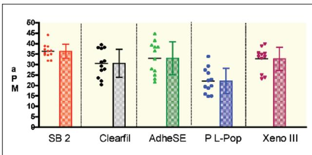
**Figure 1.** Dot Plot Graph and corresponding mean and standard deviation of the microshear data (in MPa), according to the groups.
