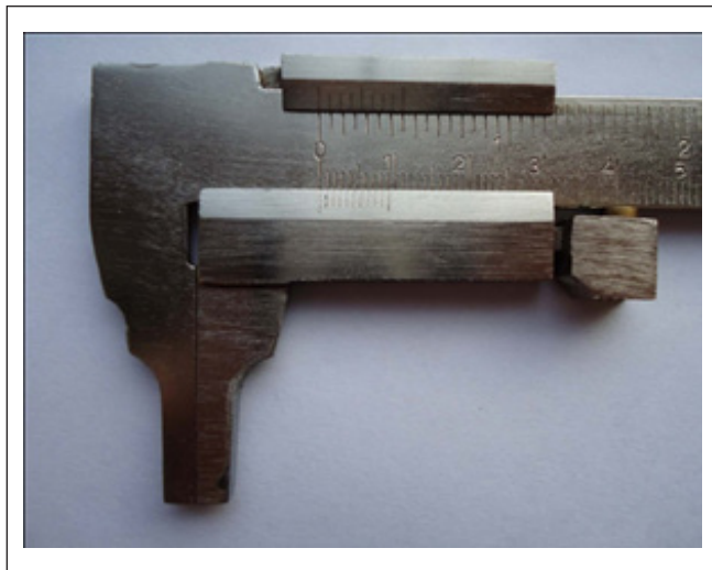
Figure 3. Modified Vernier Caliper. (Smaller jaw is removed; outer edges of larger jaw are straightened. Distance between two outer straight edges of larger jaw is 9 mm when zero reading of vernier scale and main scale coincide. Final Readings taken after adding 9 mm to the original measurement)
