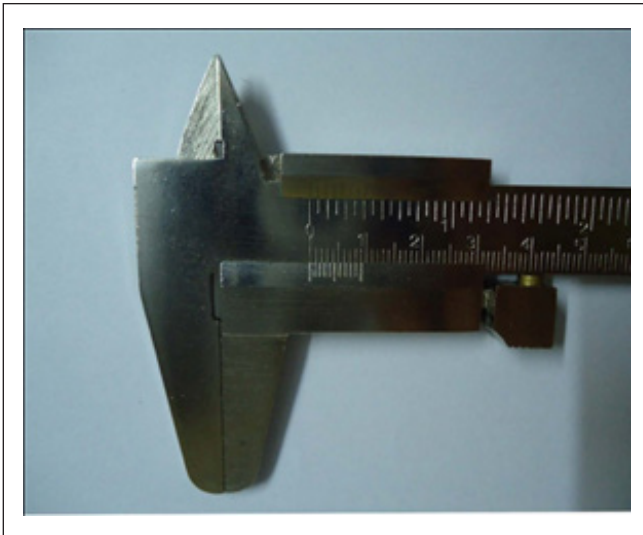
Figure 1. Vernier Caliper (Original form) comprises of two jaws, larger and smaller and two scales, vernier (sliding) scale and main scale.
