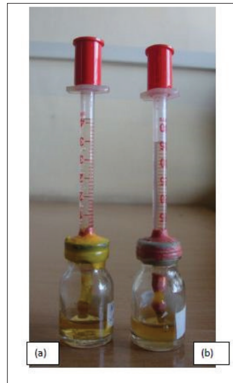
Figure 2. Bacterial leakage Model (a) Without and (b) With Turbidity
