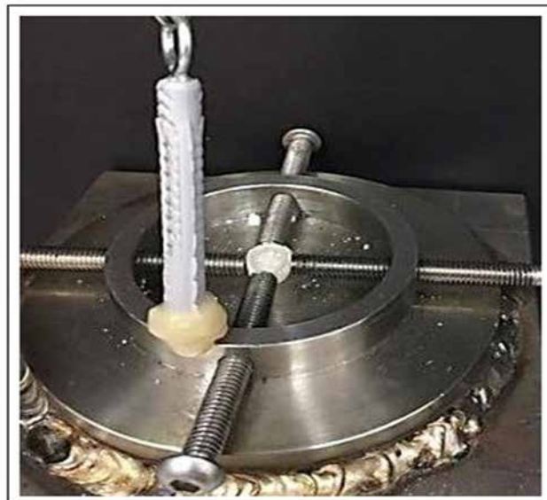
Figure 3. PPZCs dislodgment after applying tensile force parallel to the long axis of composite tooth replica.
